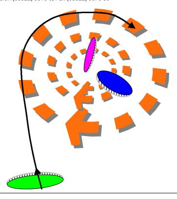
In Germany a controlled approach and landing circuit is mandatory (as on airfields) for paragliders and hanggliders. It consists of a circuit with the wind, transverse to the wind and a final approach against the wind.
