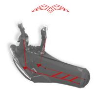
Test your speed system for the correct length of cord on the ground first (simulating flying position), with your harness and risers, before flying with it! The full range is reached when the 2 pulleys join together.
