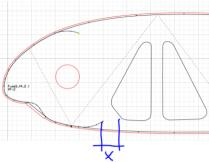
The length pf the bottom plastic rods is extended about 7% (X value in drawing above, reference to chord length).
