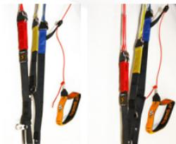
The AIRBORNE's speed system works in two parts. The transfer of the riser between the different line groups and the pulley system has a 1:3 transfer and means the AIRBORNE can use the whole range without you having to use a lot of effort. The brummel hooks on the risers and speed bar line join to the speed bar. Before launching they can easily be clipped together by a 90° turn.
