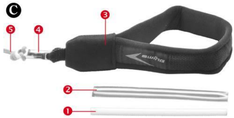
Multigrip brake handles after removing both stiffening rods. These are the various parts:
